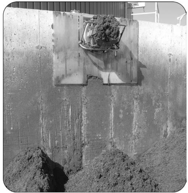
Figure 7. A manure separator connected to the anaerobic digester used to separate the solid fraction of digestate.
