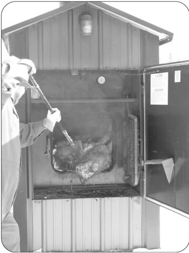
Figure 2. Improper method of incineration.
