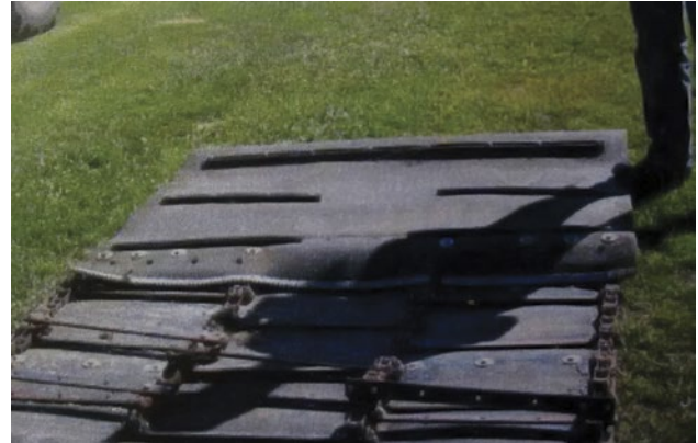
Photo 7–1. Use rubber belts to prevent plant fibre from wrapping around shafts, chains, etc. Courtesy of Manitoba government.
