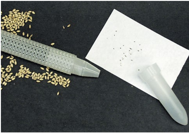
Photo 12–1. Insect probe for stored grain is inserted into grain to trap insects.
