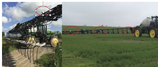
Figure 11–1. Real-time Variable Rate Nitrogen application using optical sensors mounted on a y-drop fertilizer applicator. Greenseeker™ sensors circled in red on the boom for both wheat and corn
