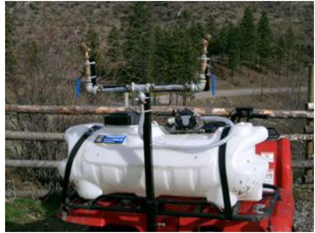
B.C. cherry grower Greg Norton's version of the same equipment. Note the independent shut-off valves for each nozzle.
