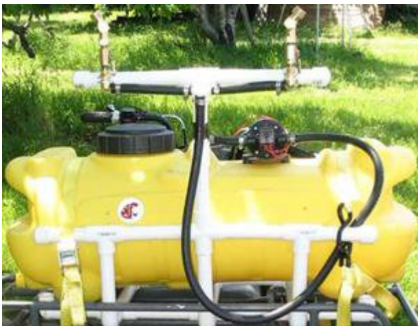
Ultra low-volume application equipment for GF-120. The frame is built from 1" PVC pipe. Photo: WSU website listed in article.
