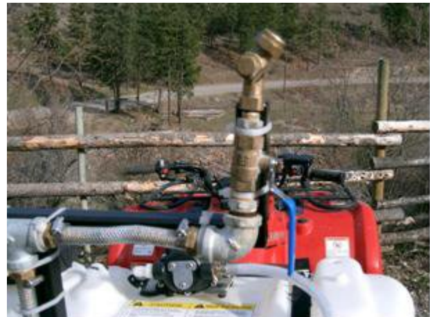
Close up of one nozzle. The swivel feature is critical to be able to properly treat different sized trees. Photo: Chris Norton.
