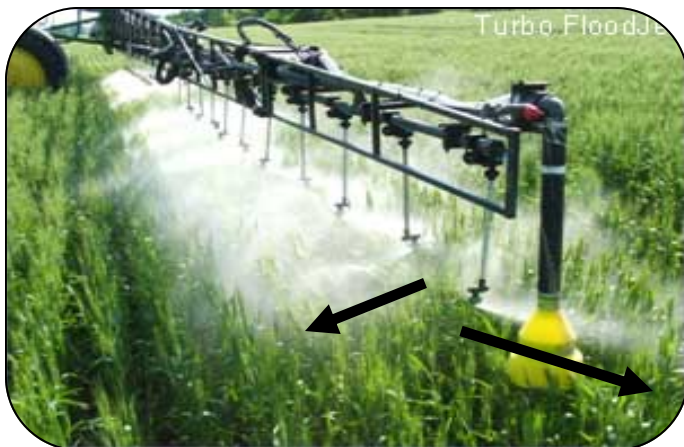
Photo 1 – Alternating Turbo Flood Jet nozzles
