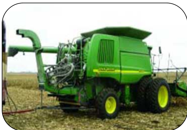
Figure 1. Modified Combine for Crop Residue Capture
