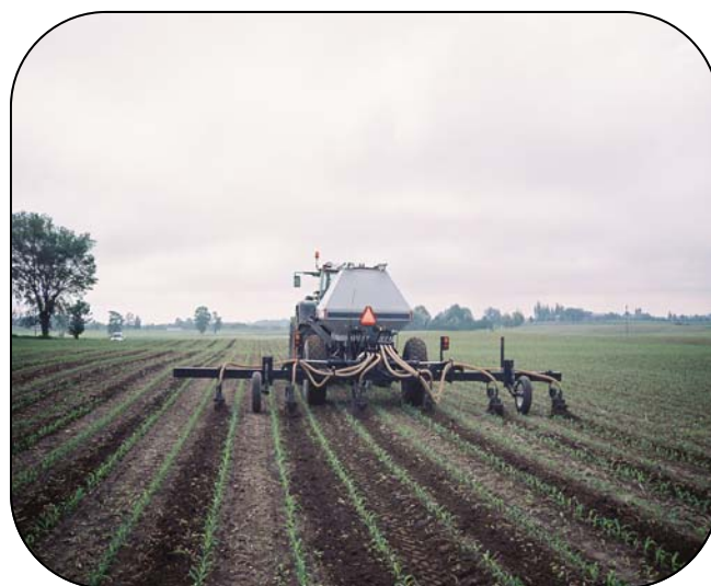
Figure 2. Claussen Farms of Brucefield Ontario sidedress urea with an air cart in their efforts to capitalize on sidedress efficiencies and the cost advantages of urea over UAN. Note the applicator bar using coulters to incorporate urea in a skip row configuration.
