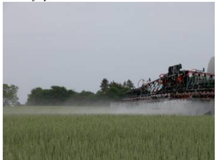
Figure 1 – Spray droplets being applied by this self-propelled sprayer may be moved off-target by excess wind speeds.
