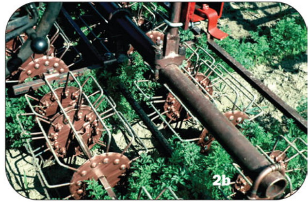
Figure 2. Two types of mechanical weeders: Torsion weeder (2a); Basket weeder (2b). (Source: Agriculture and Agri-Food Canada)
